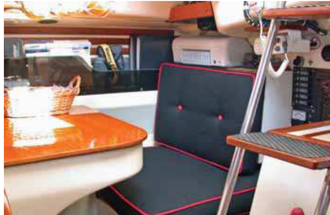
A Nav station is located on starboard, with a molded desk, hinged teak desktop, a roomy seat and a cabinet behind the backrest. A shelf alongside holds binoculars, flashlights and books for navigation.
