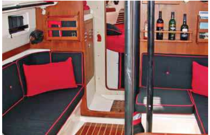
A dining table rides on a 2-inch diameter aluminum post, allowing it to lower to complete a double berth. Midway up the post, it's a table. High against the cabin top, as it is here, it's out of the way—opening up the salon as a sitting area.
