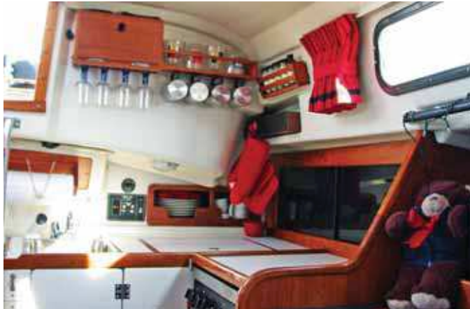
The L-shaped galley is located to port, aft of the settee. It has a nine-cubic-foot refrigerator, a deep sink and a three-burner stove with oven. It provides good space for galley needs.
