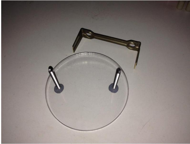
I used butyl tape to seal the plastic disc to the instrument panel to make a water-tight seal and used two more Nylok nuts to snug up. Now the digital display is out of the elements yet can be easily read from behind the wheel.
