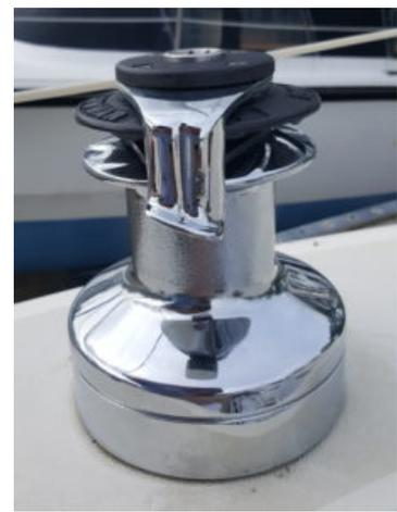
Next I cleaned the aluminum parts with a strong acidic cleaner. Lastly I painted all the aluminum parts which do not come in contact with line using a flat-black outdoor spray paint. I also painted the plastic top cap to match the aluminum casting. I know that the paint will deteriorate with time, but the gorgeous drums just didn't look right with the 'natural' faded-and-deteriorated looking aluminum.
