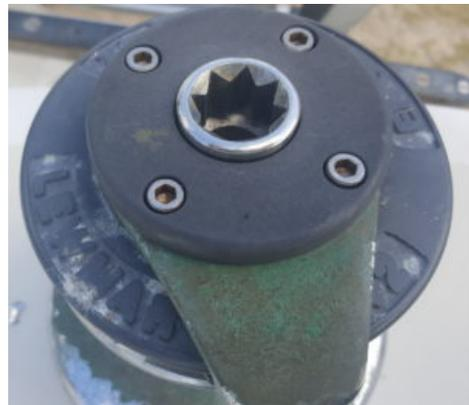
top is a molded plastic cap which holds the bronze split locks (collets) in place. Four 1/4" – 20 3/8" stainless steel socket head cap screws secure the top cap to the cast stripper arm.
