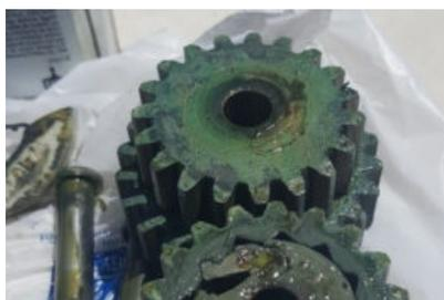
With the drum removed, I took my first look at all the moving parts inside. What a sight, it all looked like crap and the grease felt sticky like molasses or thick honey and I could not hand turn
