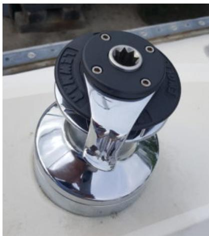
chrome platter and dropped off the drums. He glass beaded the drums (a form of sand blasting which is less aggressive) and to my surprise returned the gripping pattern to the middle of the drum. I scraped off the gross corrosion from the Aluminum parts with a small straight blade screw driver and then scotch-brighted all surfaces.
