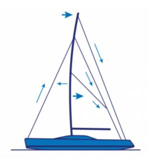
To control sag properly and independently on a fractional rig, running backstays are required.
