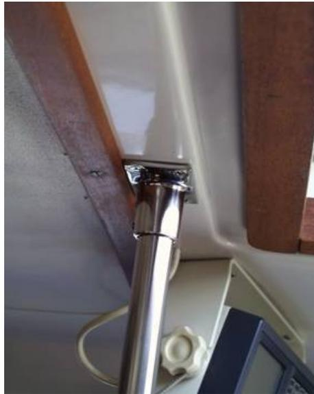
Before final installation the aluminum plate was finished with a good coating of zinc chromate to reduce corrosion.
