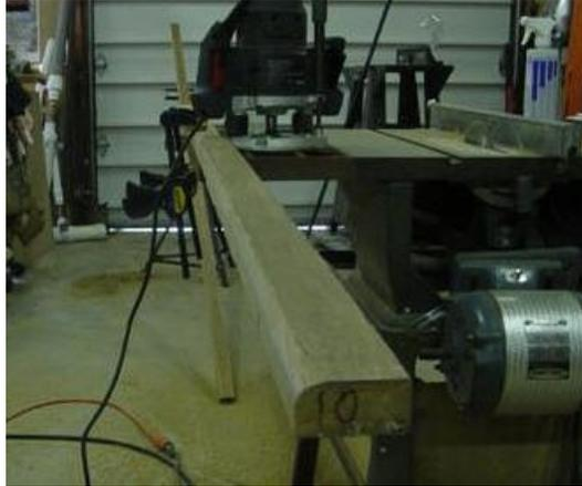
I first ripped a very thin strip off one edge of the board to square it up. Then I ripped two, 2" wide pieces.
