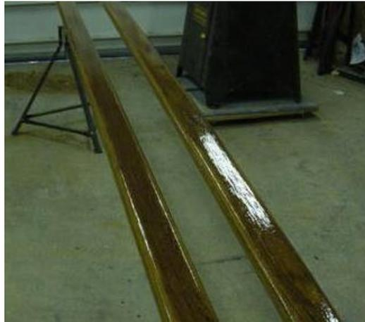
I then used a 1/2" rounding over bit with bearing in my router to round over the edges of the new rails to make them fit the hand nicely. I started out trying to use the router table, but soon discovered that my expertise was lacking and reverted to the tried and true hand method.
