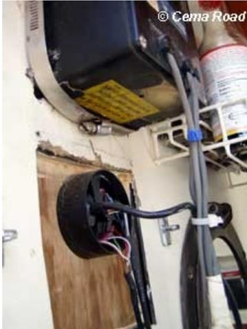
What is interesting is that the two original Signet instruments are a lot thicker than the new Raymarine unit I installed into one of the original holes. For someone doing this on their boat, the cover could be much thinner, not extending out anywhere near as far as the one on Ping.
