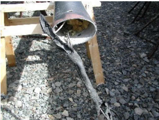
The foam in the mast is rather easy to break up and remove.
