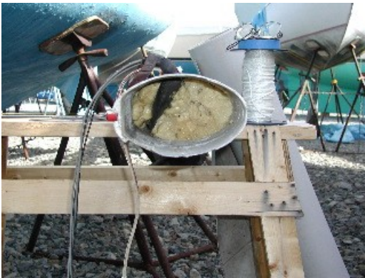
Removing foam from the bottom of the mast.
