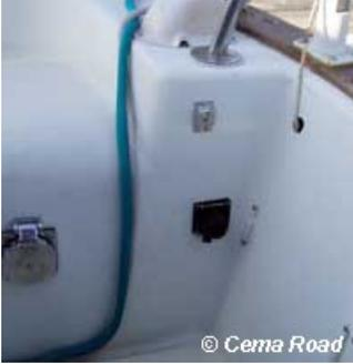
The RAM came with everything required for installation. The toughest part of the job was determining where I wanted to mount it. The optimal plan would have been to hang it off the helm somewhere, but since I had no real conduit to the helm and no NavPods installed it wasn't practical for Ping. The next best place was behind the helm on the starboard side of the cockpit, about halfway up from the sole. I'd mount the mike holder just above the connector.
