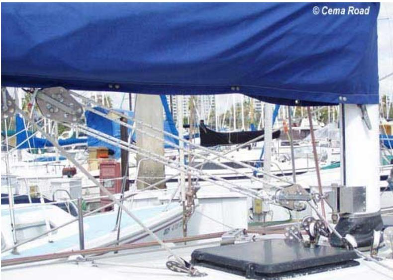
The traveler adjustment works equally as well. Lines on either side of the traveler car run to blocks on the top end of the traveler frame. They then route back to a block on the car, winding back to another block on the aft side of the traveler frame. The lines from both sides then snake to two turning blocks just to port of the companionway hatch and ahead of the dodger. Their journey ends in a pair of cam cleats at the edge of the cabin top.
