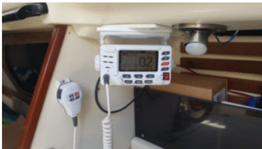
View from Nav Station (Dolly Rotated) - Internal GPS antenna picking up 12 Stats.
